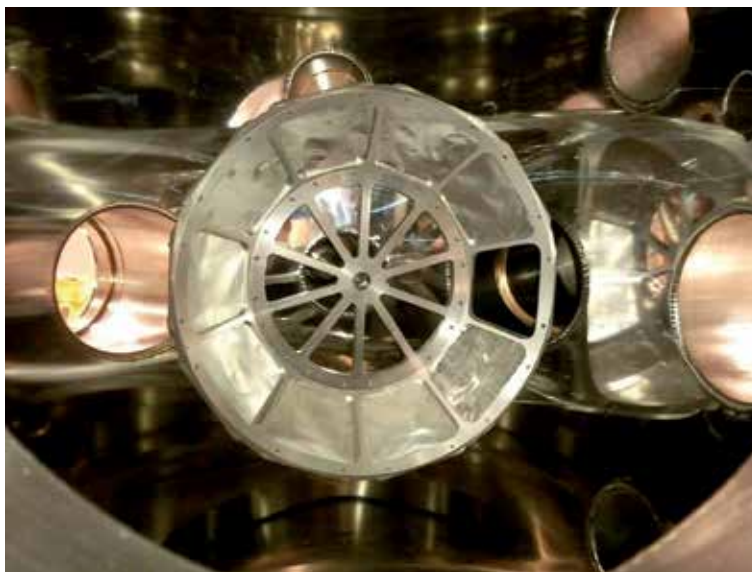
Figure 3. Umbrella shaped wheel of the beam energy degrader prototype.
