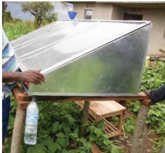
Figure 5. One of the new solar water purifier designs deployed in Uganda for consumer trials.
