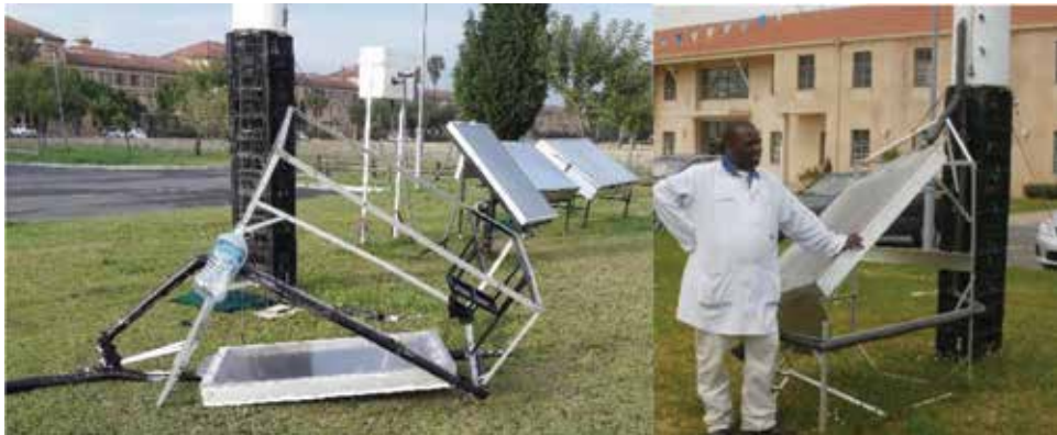
Figure 3. The blown-over solar collector (left) and the author inspecting the repaired system (right).
