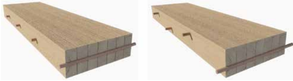
Figure 13. DLT with linear (left) and staggered (right) fastening patterns.
