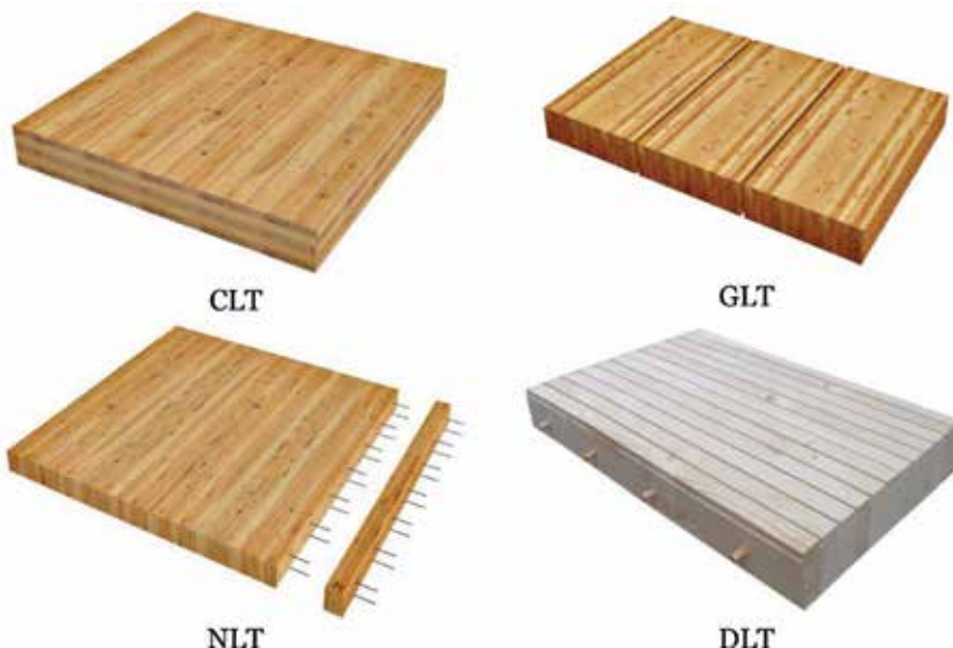
Figure 1. Lumber-based MTP (Source: Images obtained from StructureCraft).
