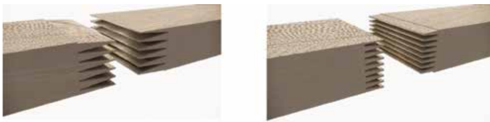
Figure 3. Two finger joint profiles (left: 29-mm long; right: 13-mm long) used for joining short pieces of lumber.
