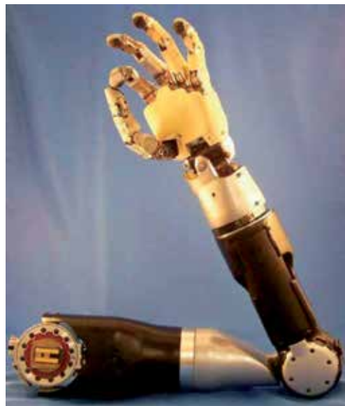
Figure 9. The modular prosthetic limb by John Hopkins Applied Physics Laboratory, USA.
