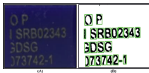
Figure 3. The detection of bounding boxes of letters: (a) text area selected; and (b) detection of letters.
