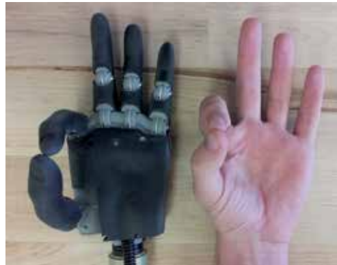
Figure 10. Third-generation Vanderbilt hand by the Center for Intelligent Mechatronics.
