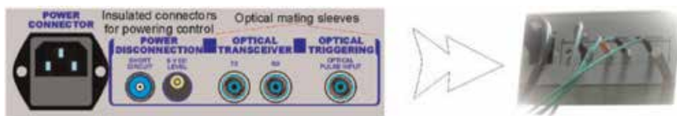
Figure 4. Elements of mobile measuring stands used for powering management and optical communication [19].
