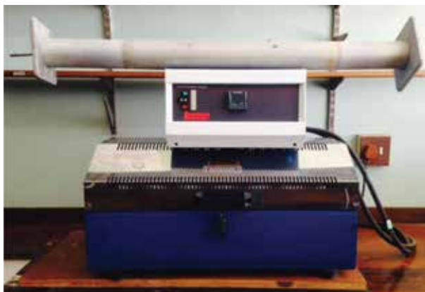
Figure 4. Image of the split tube furnace and aluminum reactor used in the fabrication of ZnO nanostructures.
