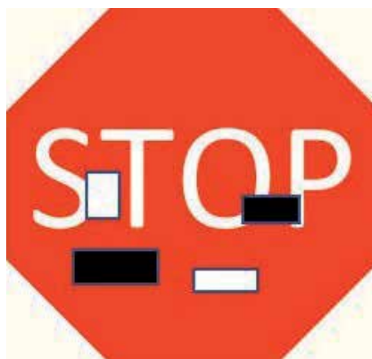
Figure 2. A stop sign with camouflage art attack (reproduced based on figures in Table 1 of [18]).
