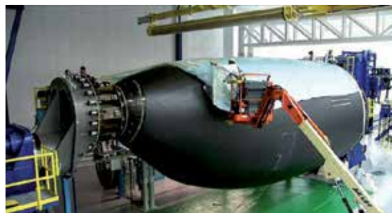
Figure 17. OML sector panel tool. Source: Premium Aerotec.
