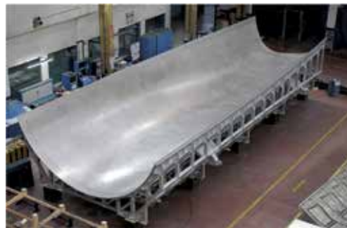
Figure 17. OML sector panel tool. Source: Premium Aerotec.
