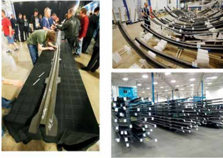
Figure 36. A350 precured omega stringers. Source: Deseret News, Jeffrey D. Allred; CW/Photos: Jeff Sloan.
