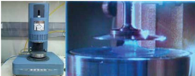
Figure 13. AR 2000 rheometer and parallel plates [56].
