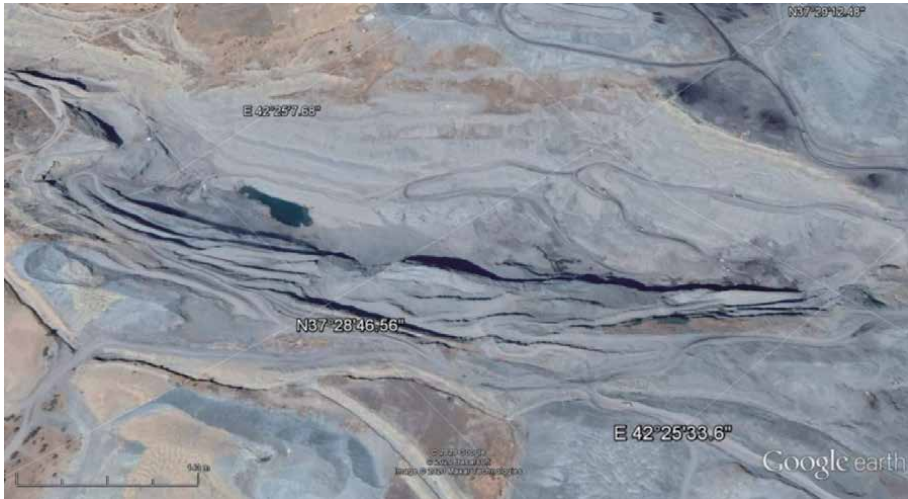
Figure 16. Open pit mine No.2: excavations for steep slopes— asphaltite excavation.
