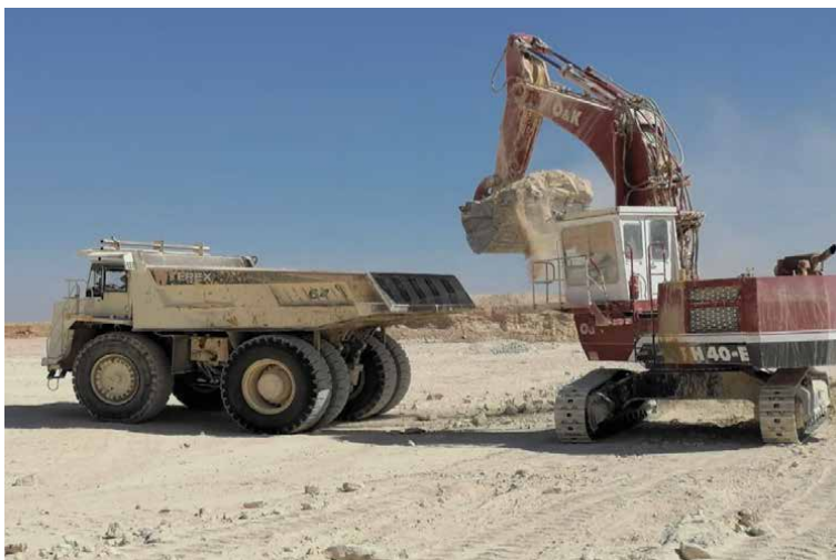
Figure 29. During loading A1 phosphate layer at Al-Shidiyah phosphate mines.
