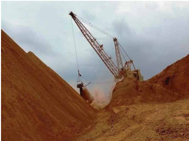
Figure 30. Dragline removes overburden at Al-Shidiyah phosphate mine, Jordan.
