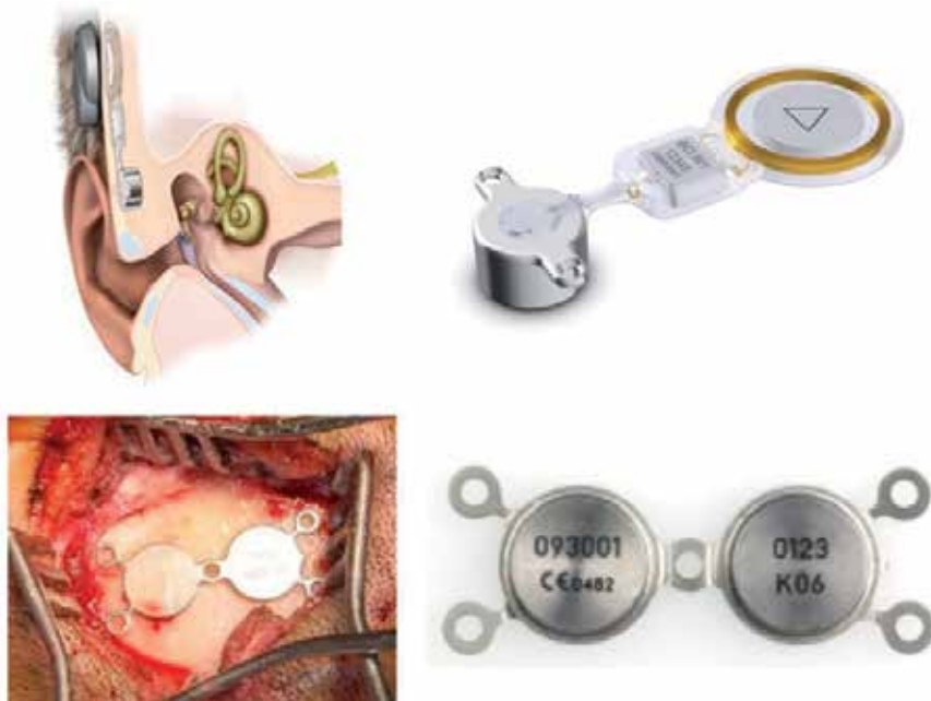
Figure 5 On the top of the image, a semi-implantable transcutaneous device BONEBRIDGE (Medel) and on the bottom another model of transcutaneous BAHI ALPHA 2 by SOPHONO (Medtronic).
