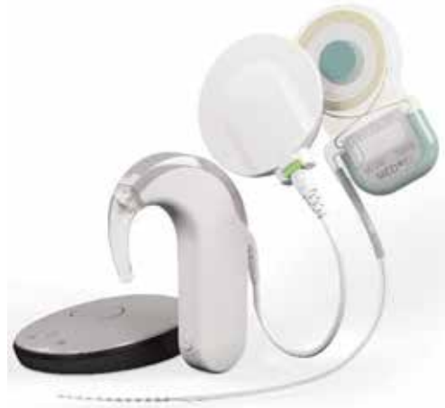
Figure 4. Image of a cochlear implant showing the implanted and externally worn audio processor parts (behind-the-ear audio processor and single unit audio processor (courtesy of MED-EL GmbH).
