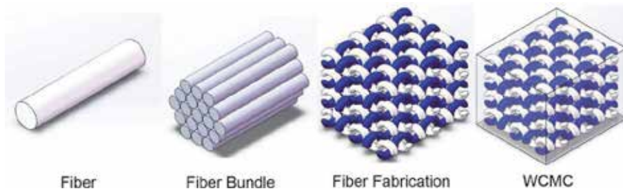
Figure 1. The fabrication process of an WCMC.
