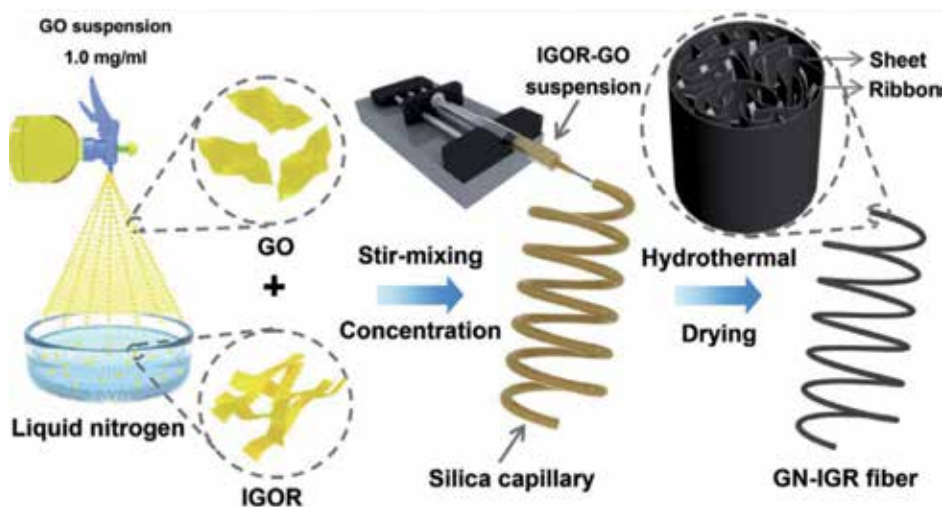
Figure 10. Schematic illustration of graphene hybrid fibers prepared by hydrothermal method [120].
