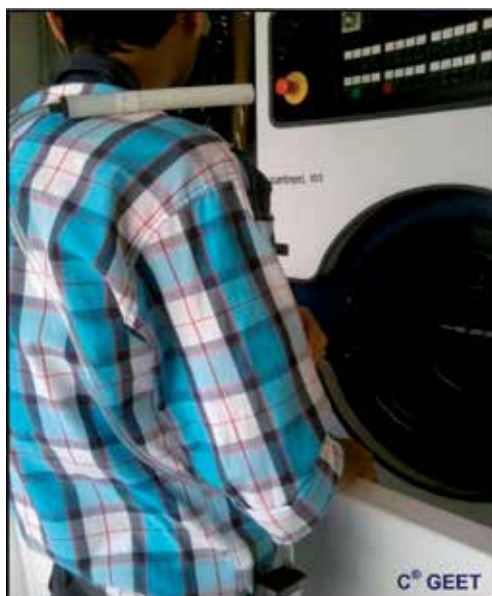
Figure 2. Active air monitoring using personal sampling.
