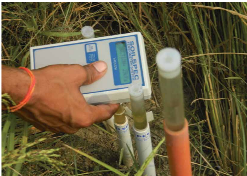
Figure 6. Soil spec in action measuring soil matric potential [20].
