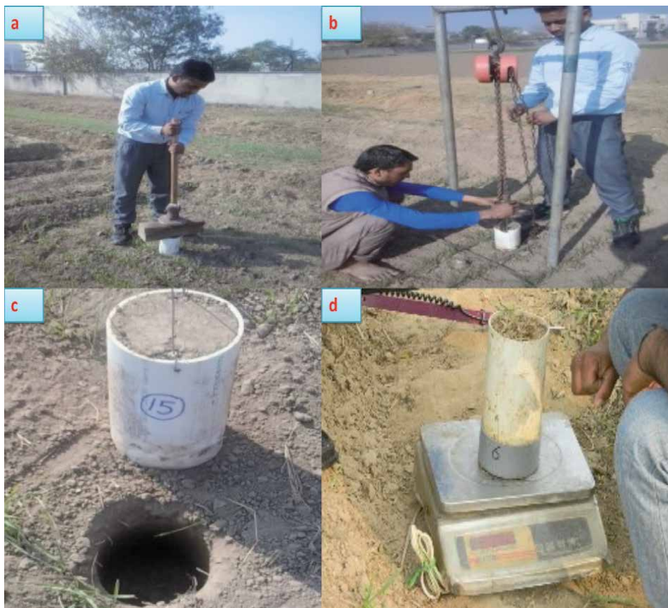
Figure 9. Step-wise technique of evaporation delineation with mini-lysimeters (a) Fitting of lysimeter in experimental plot, (b) use of chain-pulley for removing it from plots, (c) removed lysimeter, (d) weighing of lysimeters within the plots receiving differential treatments [23].
