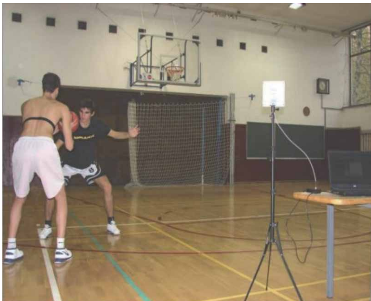
Figure 12. A powerful antenna directly connected to the computer allows measurement at a distance of up to 200 m, and the transmission and storage of data on the computer.
