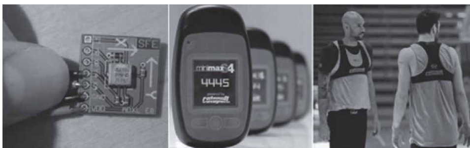
Figure 5. An accelerometer (left), MinimaxX S4 wearable tracking device (middle), and example sports vest (right). Web source: http://elite-perf.com/ .
