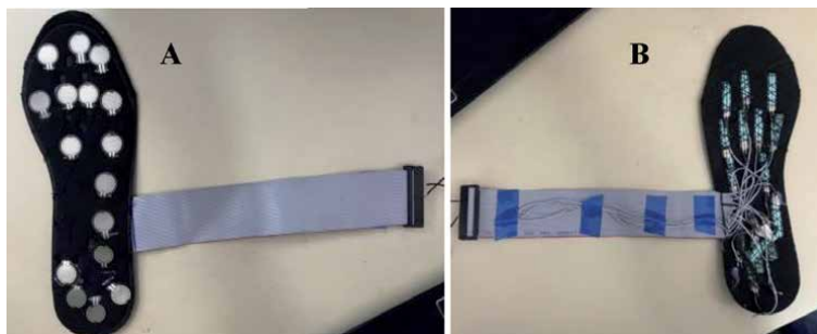
Figure 4. FSR-based smart insole: top (a) and bottom (b).
