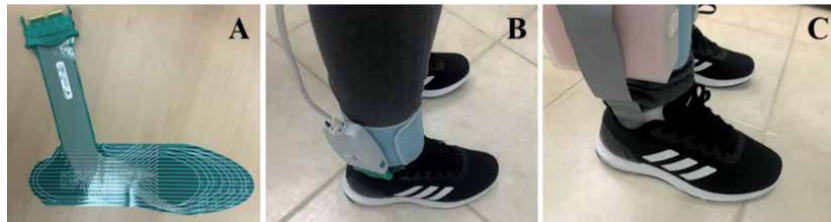
Figure 6. Comparison F-scan smart insole (a), subject 01 is wearing the F-scan system (b), and FSR-based prototype system (c).
