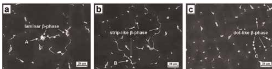
Figure 14. SEM images of the \beta -phase in as-cast ZK60 alloys (a) without ultrasonic treatment; (b) with 1200 W SUF treatment; and (c) with 600 W DUF treatment.
