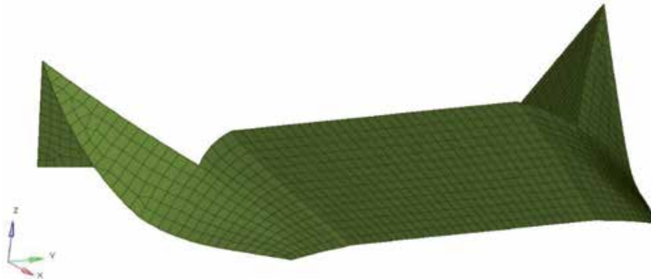
Figure 3. Sub-frame—Pure structure. The geometry was also conceived using a topology optimization algorithm just for this study.
