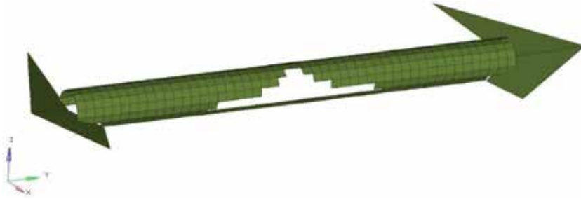
Figure 2. Torsion axle—High displacement structure. The geometry was conceived using a topology optimization algorithm just for this study.
