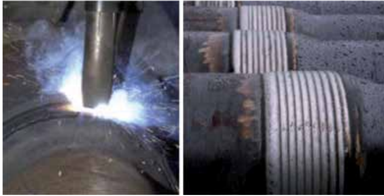
Figure 1. Hardbanding welding process and morphology after welding [1].
