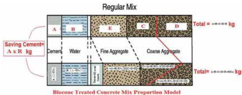
Figure 8. Concrete job mix between original mix (NFA mix) vs. modified Bioconc-treated concrete mix.
