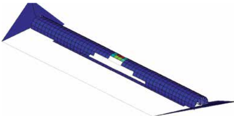
Figure 12. Frequency domain modal superposition damage result plot. Maximum damage = 68.
