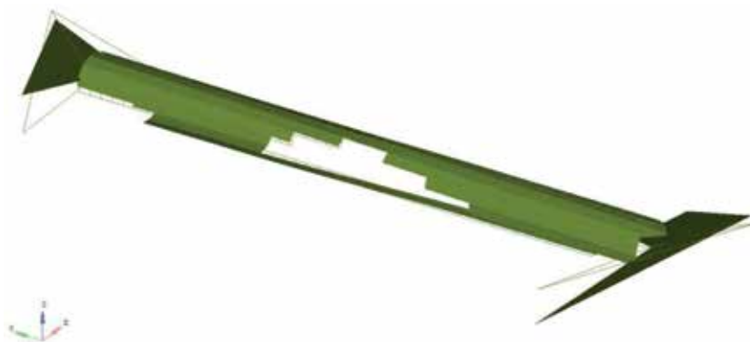
Figure 5. Torsion axle: First normal mode of 33 Hz.
