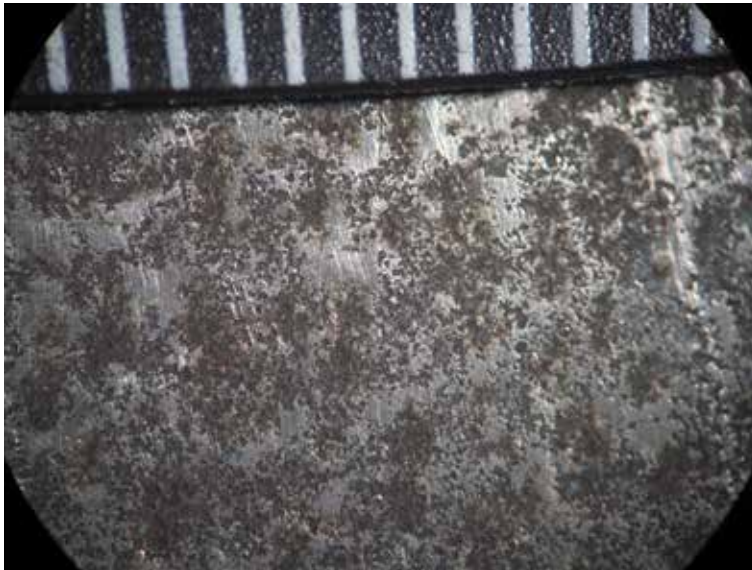
Figure 5. Typical morphology of pitting.
