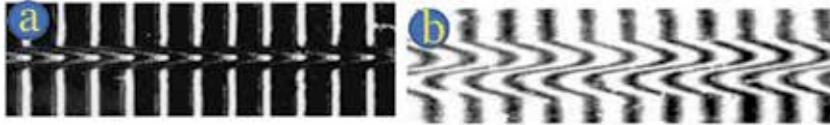
Figure 7. (a) Pluta duplicated image of LDF GR-IN optical fiber and (b) Fizeau interferogram of the same sample. Reference [50] with permission.
