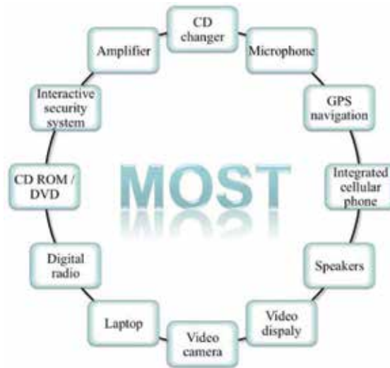
Figure 1. SI-POF-based ring topology of a MOST system in a car.
