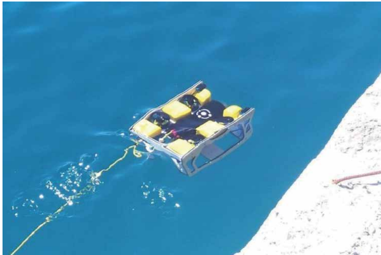
Figure 1. Equipment used SIBIU PRO (NIDO ROBOTICS): Maximum depth of 300 meters.
