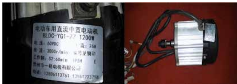
Figure 2. Three-phase synchronous motor for vehicle traction and its nameplate.
