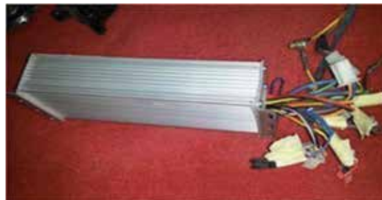
Figure 4. The DC to three-phase voltage inverter used.
