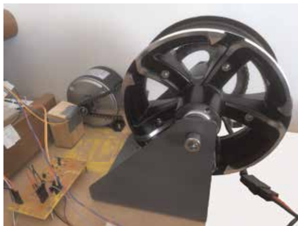
Figure 1. Suspended wheel attached to the traction motor by a crown-chain-pinion.
