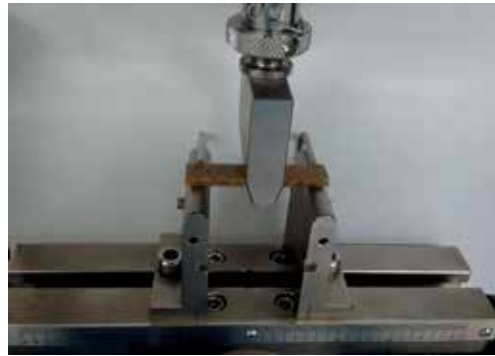
Figure 2. Assembly used for flexural test (according to ASTM D790).
