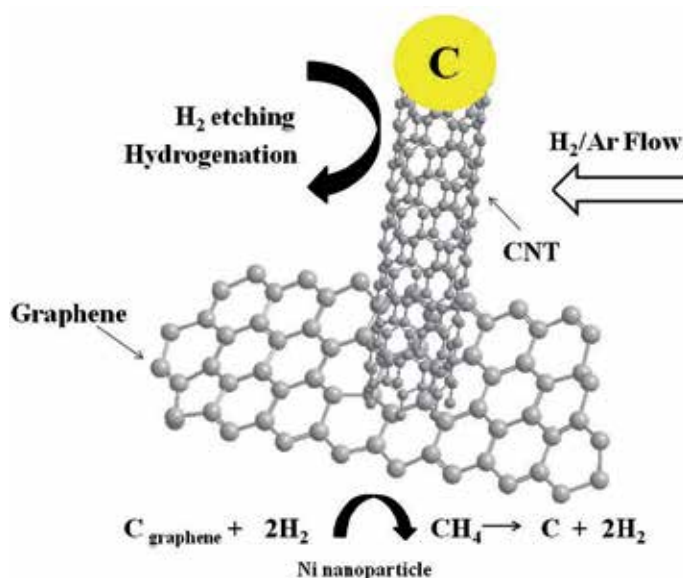
Figure 6. Schematics illustrating direct CNT growth on planar graphene under H 2 etching.
