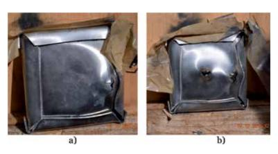
**Figure 17.**HEA-steel ballistic package during dynamic tests (a) after the first firing and (b) after the second firing.
