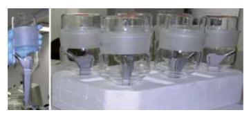
**Figure 17.** *Glass reactors for cation extraction tests.*
