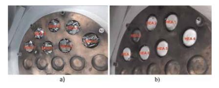
**Figure 1.**HEAB 1 to HEAB 7 batches prepared for melting on the copper plate of the RAV equipment (a) and after melting (b).
