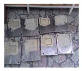
**Figure 2.** *Metallic molds for casting Al<sub>0.8</sub>CrFeCoNi alloy.*
