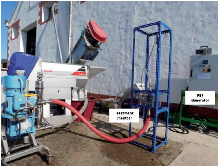
Figure 9. PEF experimental unit to process the crushed grapes at a flow of 3 t/h to improve the polyphenols extraction in the maceration-fermentation stage of red winemaking.
