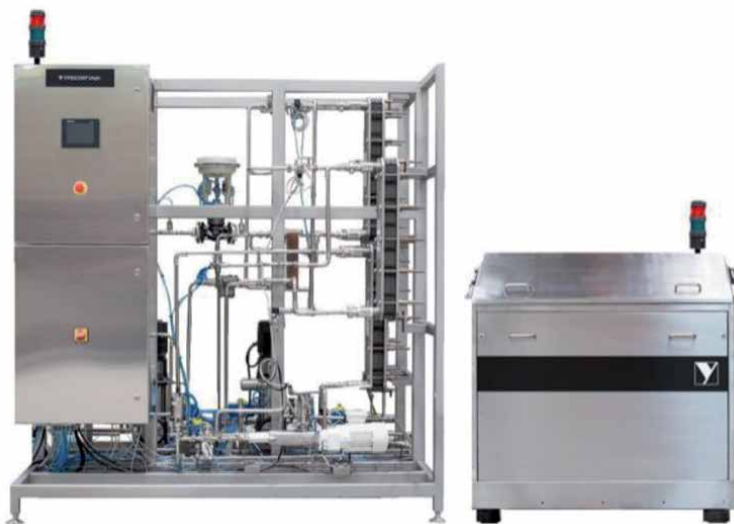
Figure 6. UHPH industrial machine (Ypsicon [28]).
