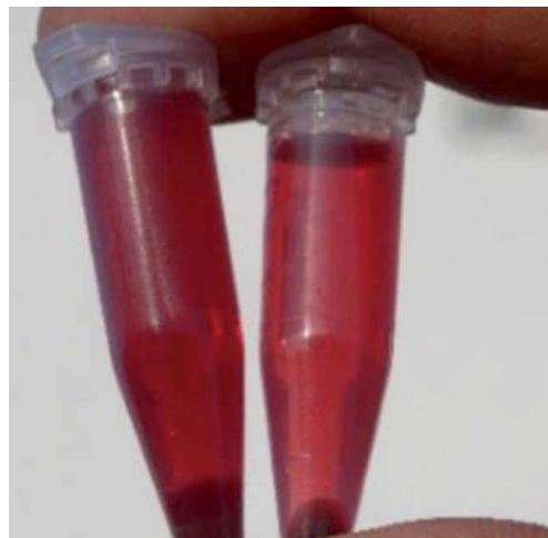
Figure 8. Color intensity and degree of pigment extraction in musts obtained from untreated (right) and PEF-treated (left) grapes ( V. vinifera L. cv. Garnacha) after 1 h of maceration.
