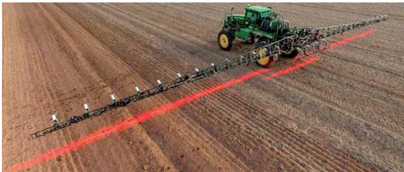
Figure 12. WEED-IT performing application with weed detection by infrared sensors. Source: SmartSensing [34].
