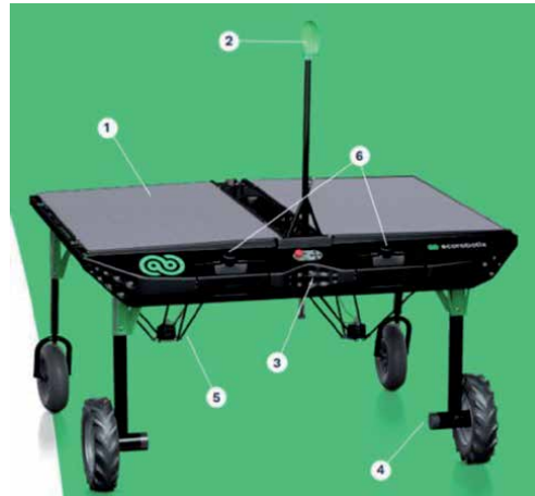
Figure 21. Ecorobotix components. (1) Photovoltaic panels, (2) camera and artificial vision for steering and detection, (3) navigation by GPS and sensors, (4) electrical drive system, (5) rapid robotic arms with sprayers, and (6) tanks for two different products. Source: Ecorobotix [45].
