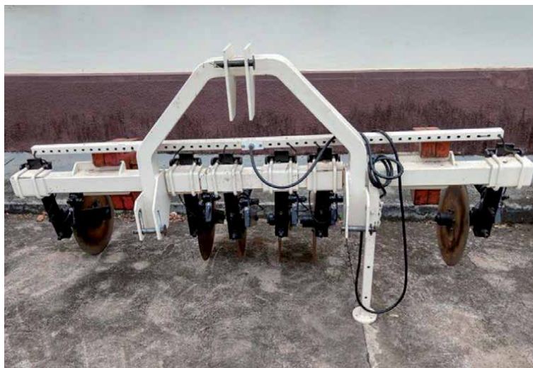
Figure 5. Veris Platform® 3100 to measure the electrical conductivity of the soil. ESALQ/USP, Piracicaba, SP, Brazil.
