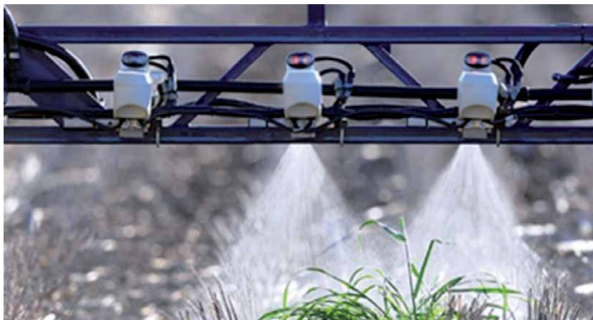
Figure 17. WeedSeeker spray nozzles applying herbicide only to weeds. Source: Trimble Agriculture [35].
