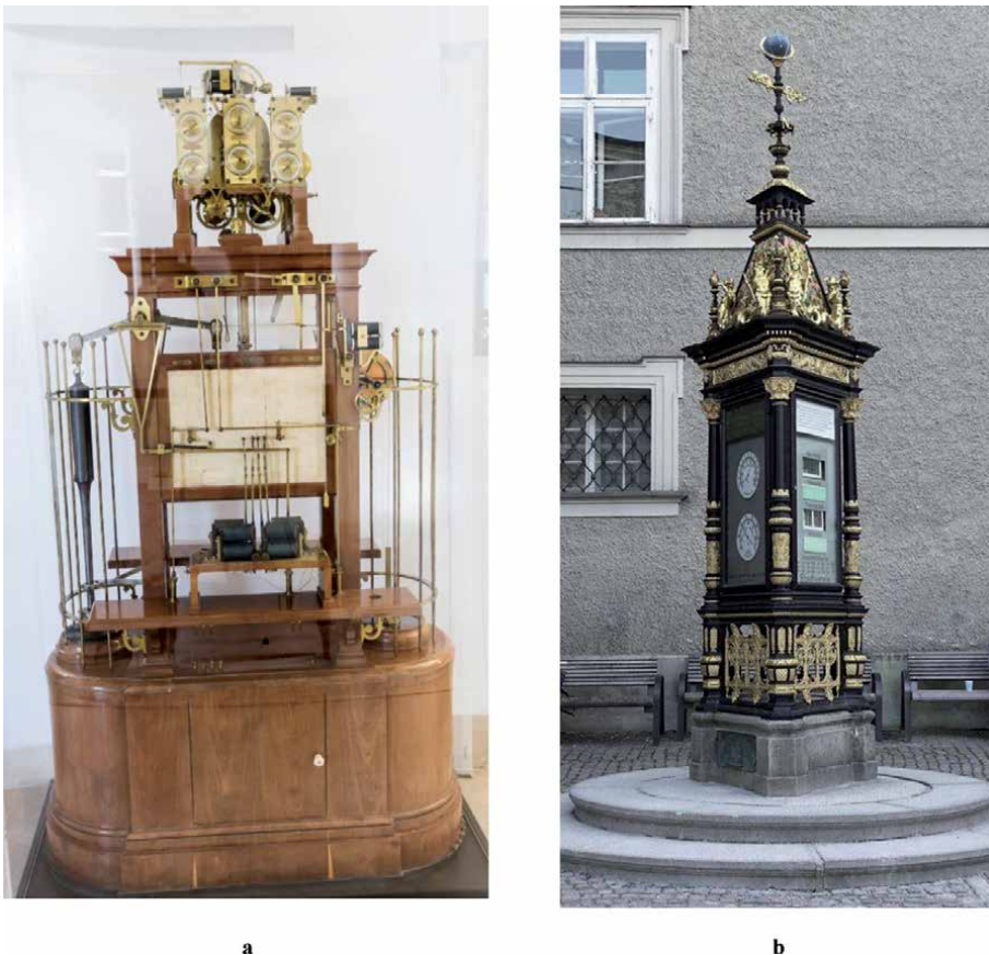
Figure 4. (a) The Meteorograph designed by father Secchi [53], and (b) the first (19th century) weather station in Salzburg, Austria.
