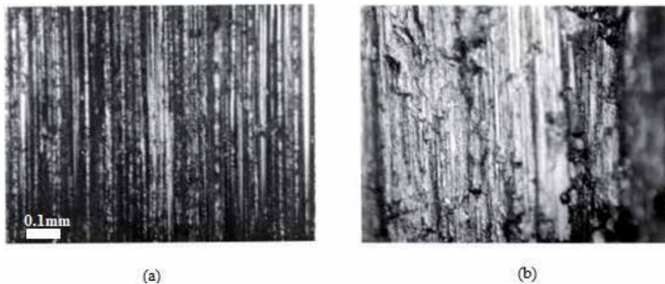
Figure 5. Optical microscope images of wears of lower specimens: (a) B and (b) D in Figure 4 [1].
